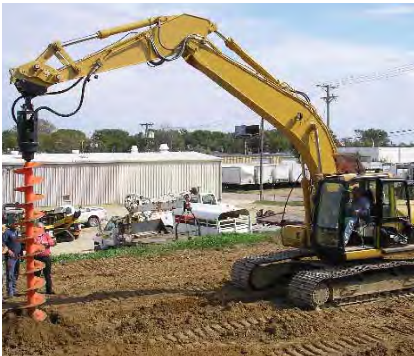
Excavator quick coupler mount used with DT-15 Drive and auger.
